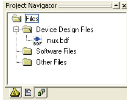
**Figure A.10** Files associated with a project as shown in the Project Navigator window.
