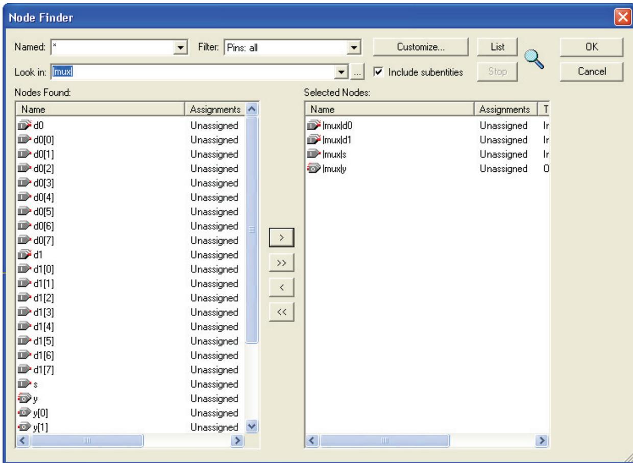
**Figure A.12** The Node Finder window for adding input and output signals for simulation.
