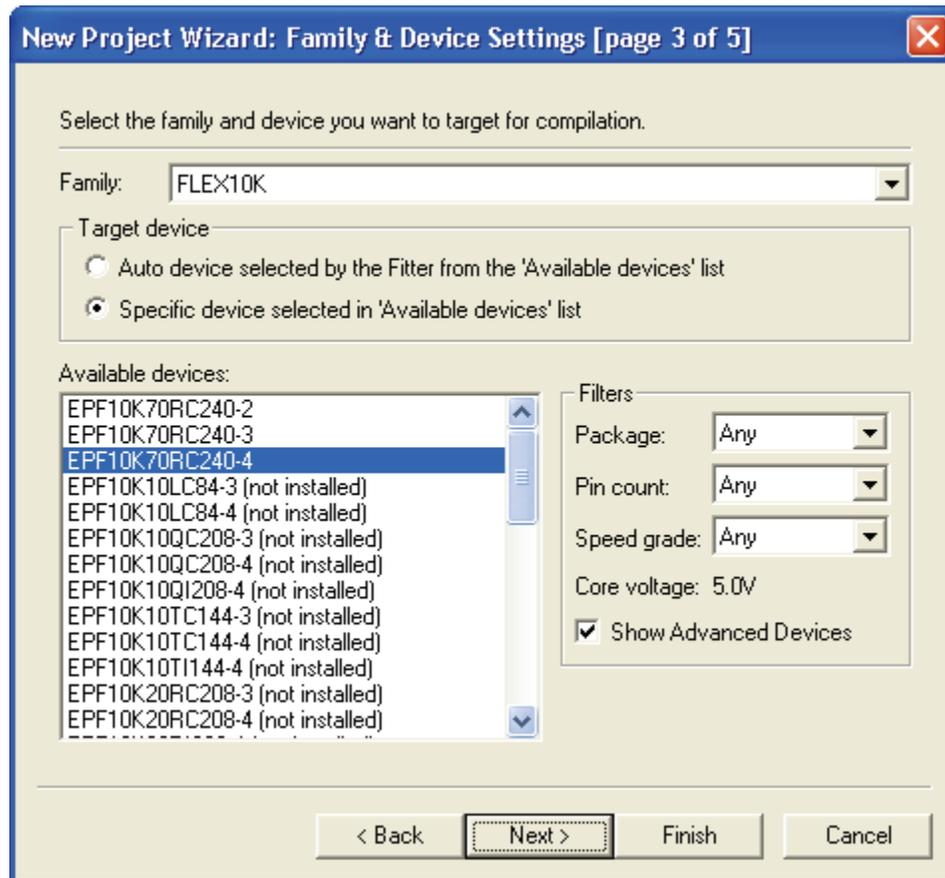
**Figure A.3** The New Project Wizard: Family & Device Settings window with the device EPF10K70RC240-4 selected.
