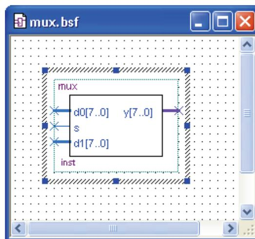
Figure A.17 Logic symbol of the mux circuit.
