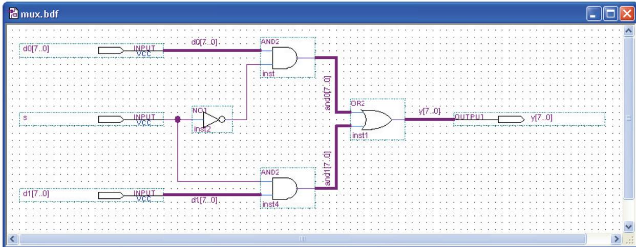
Figure A.9 Connections and names for the 2-to-1 multiplexer circuit.
