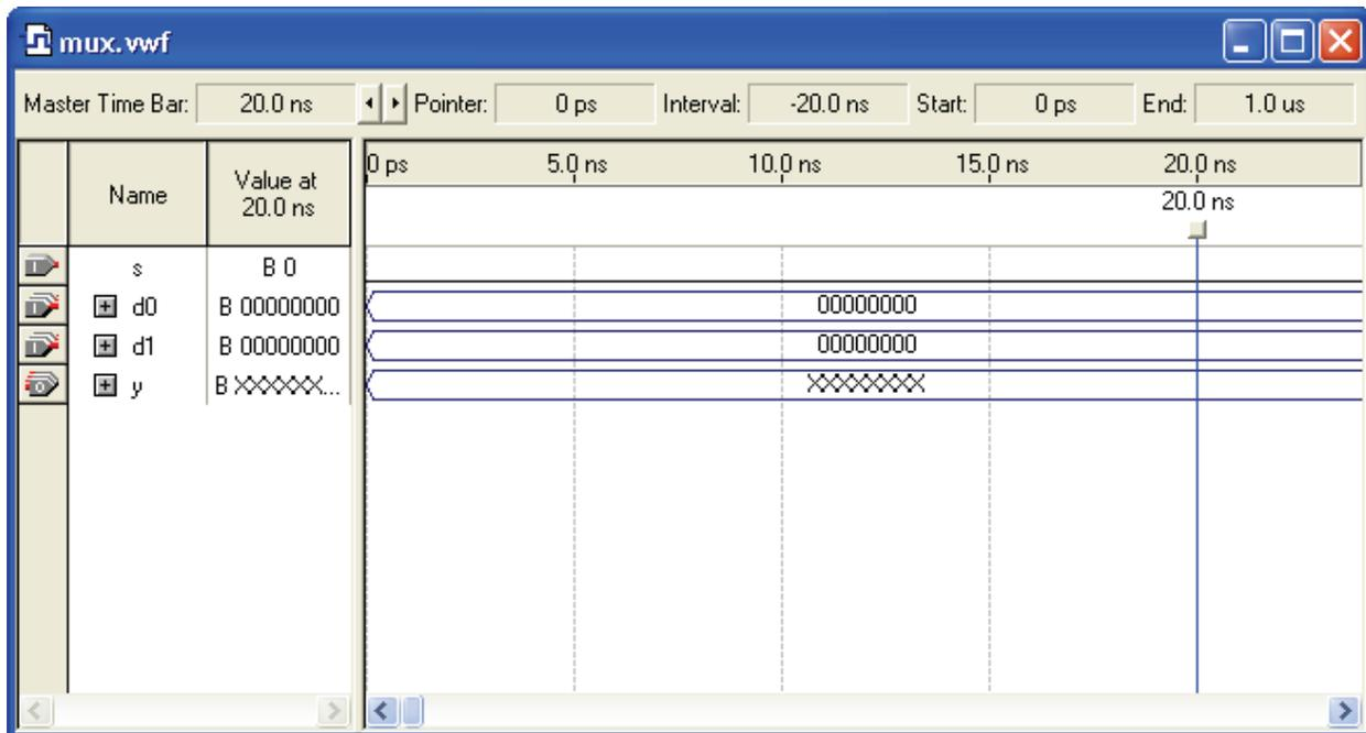
Figure A.13 The Vector Waveform window with the four signals for simulation.
