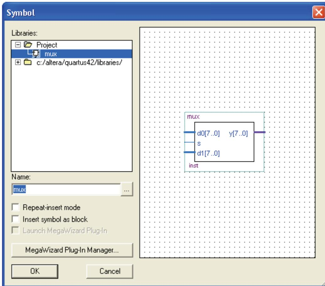
**Figure A.18** Selecting the mux logic symbol to be inserted into another circuit design.
